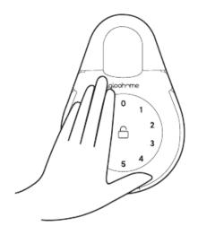
2. Key in PIN code, followed by the "Unlock Icon" in the center of the keypad
